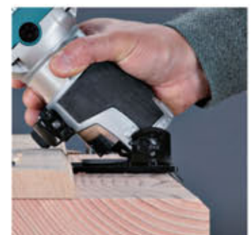
Enlarged opening section of base assembly for excellent bit visibility.
