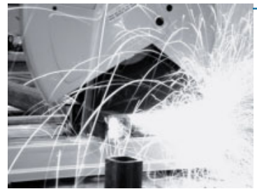
Abrasive Blades make Cuts with Sparks
