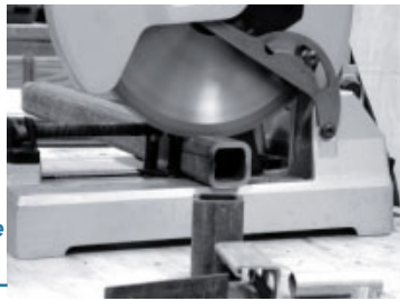
Abrasive Blades make Cuts with Sparks
