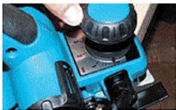
Adjustments as fine as 0.10mm can be made with the click-stop knob.
