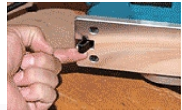
A spring-loaded parking shoe protects the cutters when you put the planer down.
