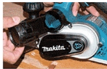
This plug can be fitted on either side of the plane to deflect shavings into the bag.
