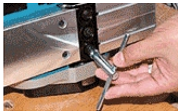
The supplied hex wrench means it's very simple to remove the cutters.
